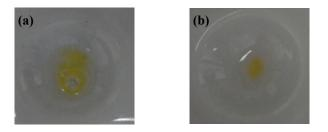
Figure 1 - Yellow-colored products of the reaction of Marquis reagent with 3,4-MDMC (a) and Liebermann's reagent with CAT (b).
