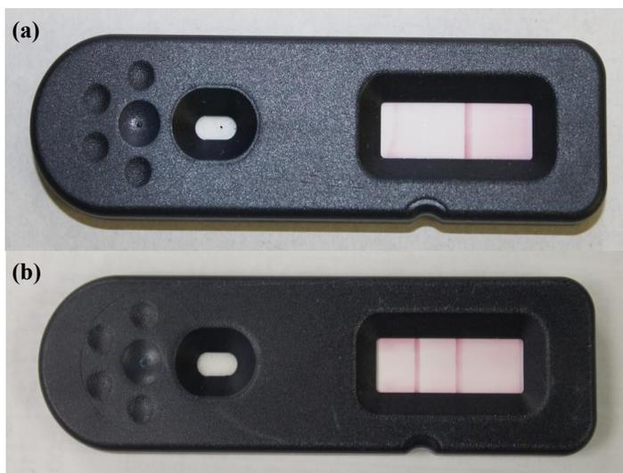
Figure 2 - Cozart<sup>®</sup> cocaine solids test: (a) Positive test for cocaine, (b) Negative test for cocaine.
