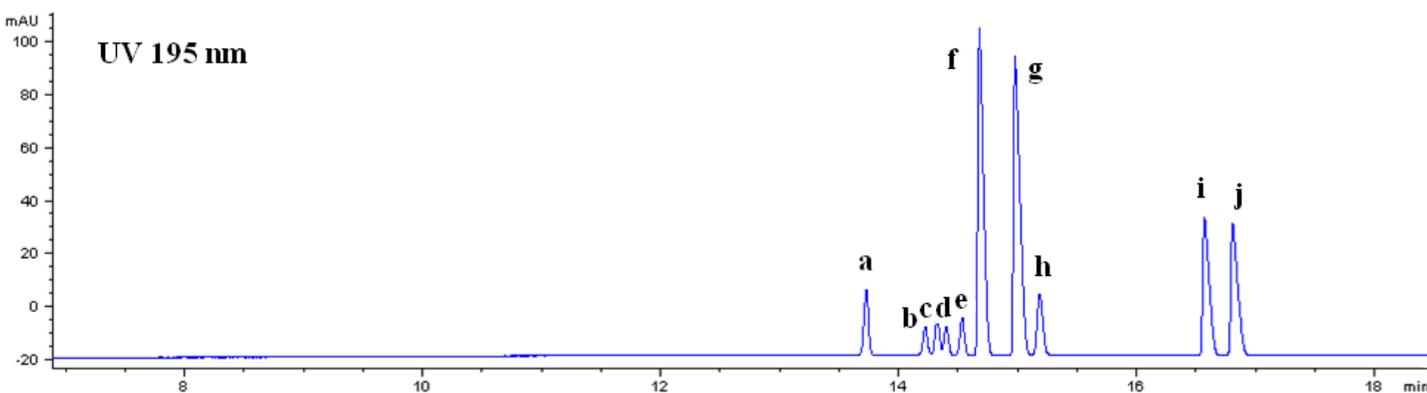
Figure 1 - Dynamically coated CE separation of standard mixture of (a) *l*-pseudoephedrine, (b) *d*-ephedrine, (c) *l*-amphetamine, (d) *l*-ephedrine, (e) *d*-amphetamine, (f) *l*-methamphetamine, (g) *d*-methamphetamine, (h) *d*-pseudoephedrine, (i) n-butylamphetamine (1), and (j) n-butylamphetamine (2). CE conditions are described in the experimental section.
