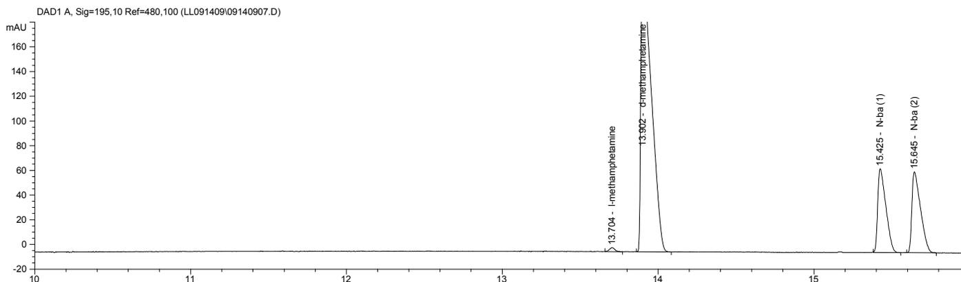
Figure 5 - Dynamically coated CE separation of methamphetamine sample containing *l*-methamphetamine, *d*-methamphetamine, n-butylamphetamine (1), and n-butylamphetamine (2). CE conditions are described in the Experimental section.
