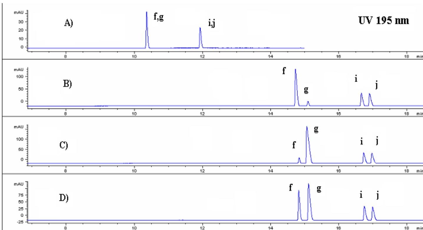
Figure 3 - Dynamically coated CE separations of methamphetamine exhibits containing (f) l-methamphetamine, (g) d-methamphetamine, (i) n-butylamphetamine (1), and (j) n-butylamphetamine (2).
